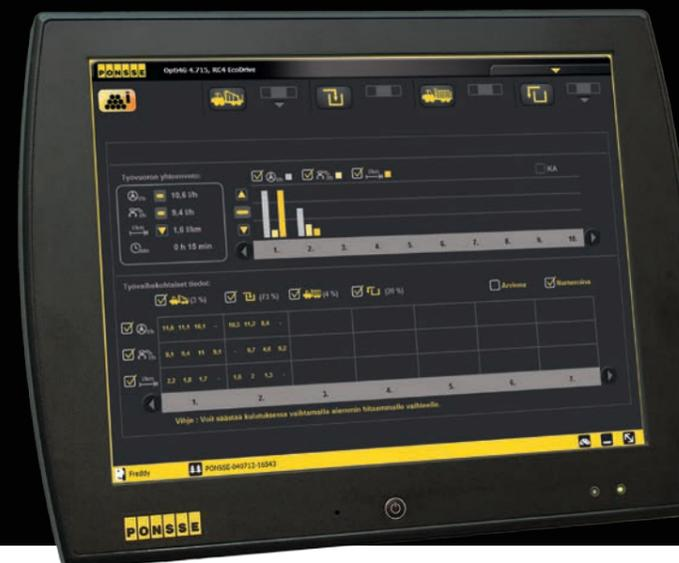
THE PONSSE ECODRIVE application provides operators with useful and easily understandable information about the use of the machine. Through the machine's control system, it monitors machine load and fuel consumption for each function and indicates in real time whether the operator's working methods and machine controls are economical and efficient. Eco-Drive lets you focus on what is essential in order to develop working methods.
