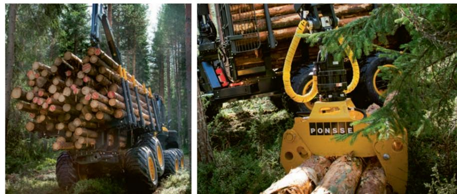
**POWER AND PRECISION** Buffalo's strong hydraulics and precise loader control enable easy and secure loading operation. The loaders have a maximum reach up to 10 m (33 feet).
